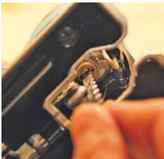
▲ Fitting the blade is very easy; you push it directly into the slot
